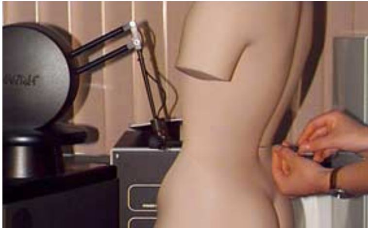
Figure 1. A lumbar puncture needle (attached to the haptic device) is passed through a human mannequin torso.
